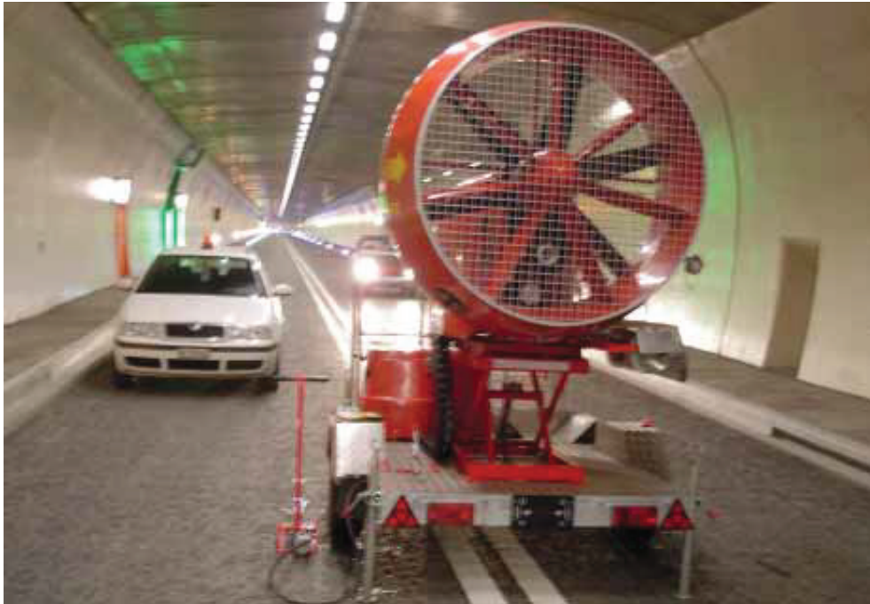
Figure 5: Mobile jet fan
